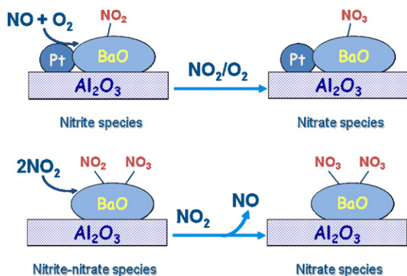
Fig. 2. Reaction pathway for NO x adsorption over Pt-Ba/γ-Al 2 O 3 catalysts.
